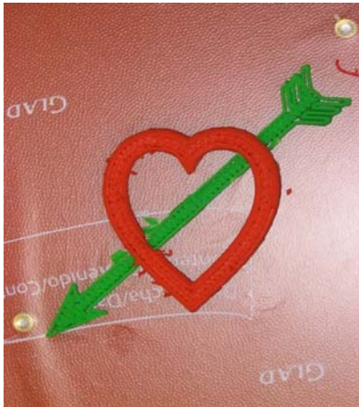
Figure 5 – The green arrow extends fully through the heart, and the red frosting is printed right over it, creating an integrated structure.
