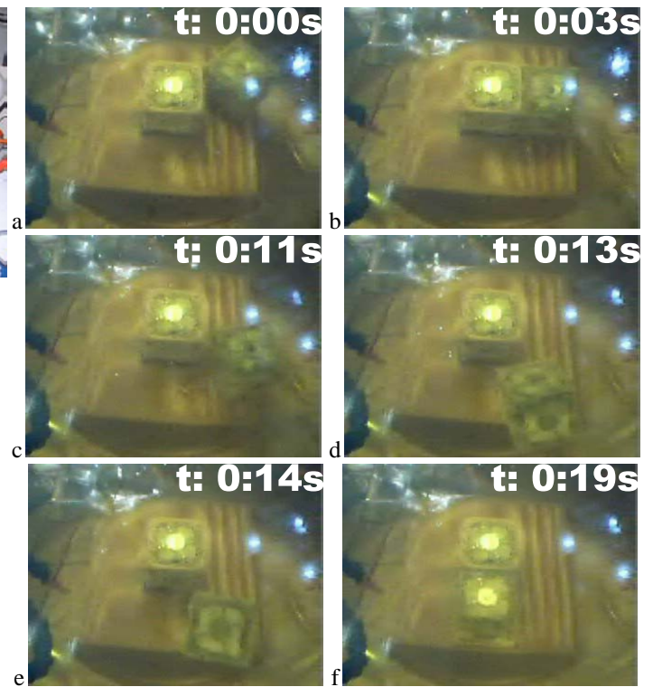
Fig. 5. Physical self-assembly and reconfiguration using magnets for bonding. The anchored unit attracts a free-floating block (a), which then attaches and bonds to the anchored block, demonstrating self-assembly of a two-unit structure (b). The second unit is then rejected, but the rejection, in addition to random fluid agitation, brings the unit close to a different face (c-e). The unit then re-attaches, resulting in a new two-unit structure, thereby demonstrating self-reconfiguration (f).
