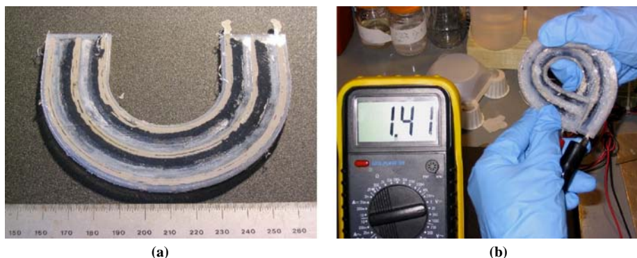
Figure 9 (a) Freeform-fabricated two-cell zinc-air battery with unusual geometry; (b) partial functionality is retained while the battery is deformed
